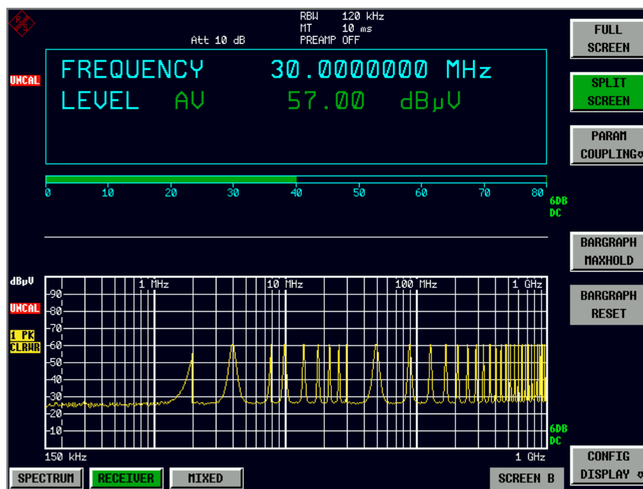
Fig. 4.16 Typical split-screen display
